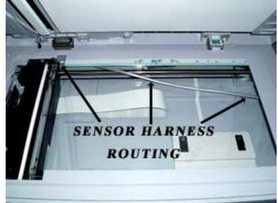
As you can see, the routing for this application is much simpler on this particular copier. The routing will vary from copier to copier, but the principles of allowing for enough slack and not interfering with the movement of the light bar, and the harness not interfering with the light path remain the same on all devices.
